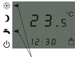
Arrows displaying the current operating status
